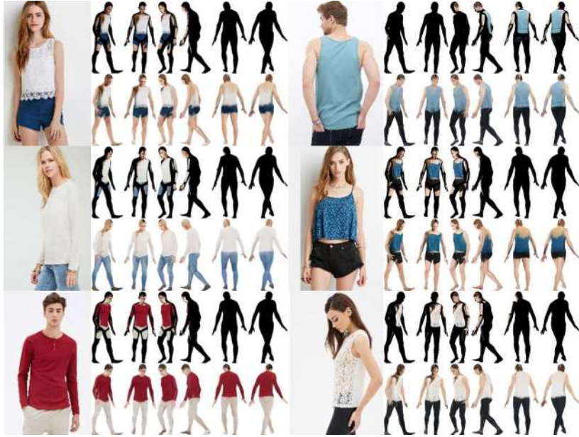
Fig. 3. Warping module results. For each sample, the top row shows interpolated textures obtained from DensePose predictions and projected on the surface of the 3D body model. The bottom row shows the same textures after inpainting in the UV space.
