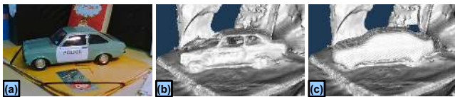
Figure 4. Reconstruction with specularities and transparent surfaces: (a) scene, (b) reconstruction without priors, (c) reconstruction with priors.
