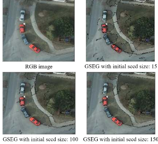
Figure 4. Illustrations of GSEG segmentations with different initial seed sizes: \tau = 15, 100, 150 .
