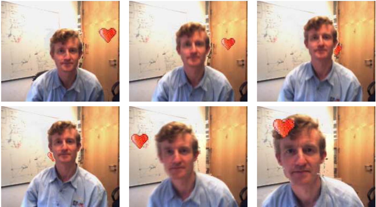
Figure 31: Inserting 3D emoticons. The proposed algorithm generates depth information together with new synthetic views. The estimated depths can be used for convincing insertion of emoticons in the 3D space. This figure shows some cyclopean views generated by our algorithm where a rotating “emoticon” has been inserted. Notice that in the 3 rd and 4 th images the emoticon heart is half occluded by the neck of the person, thus demonstrating correct handling of occlusion events. The two left and right input sequences are not shown here.
