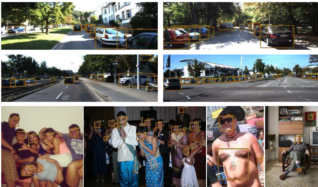
Figure 7: Examples on both the MALF detection set and KITTI car detection set. The numbers above the bounding boxes are the confidence score. Our system works very well in complex scene where objects are small and highly occluded. However, it still could miss some objects and generate false alarm.
