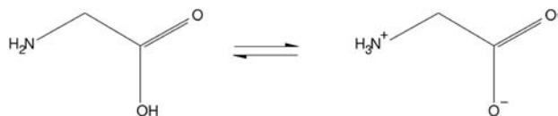
Figure 3. Equilibrium between neutral glycine (left) and its zwitterionic form (right).
