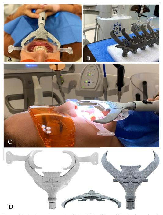
**Figure 3.** 3D printed aerosol interception device. (**A**) Frontal view of 3D printed aerosol suction attached to surgical suction system and oral retractor. (**B**) With 3D printing, each office can be supported with adequate quantities. (**C**) Lateral view of "SUR-FACE" attached to conventional retractor. (**D**) View of "SUR-FACE" with and without cheek retractor and view of three suction openings.
