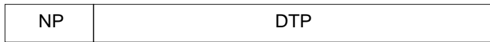
Fig 59. An example of time-division system. The shared channel time is divided into superframes (SF) and further divided into a network control part (NP) and a data transfer part (DTP). Sometimes, the duration of the NP depends more on the number of the associated devices than on the amount of information broadcast there.
