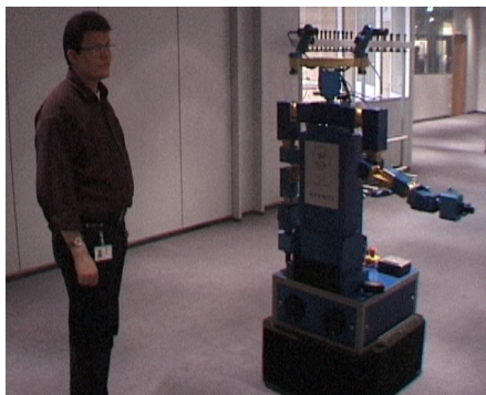
Figure 1: HERMES describing the way to a location of interest via voice and gestures
