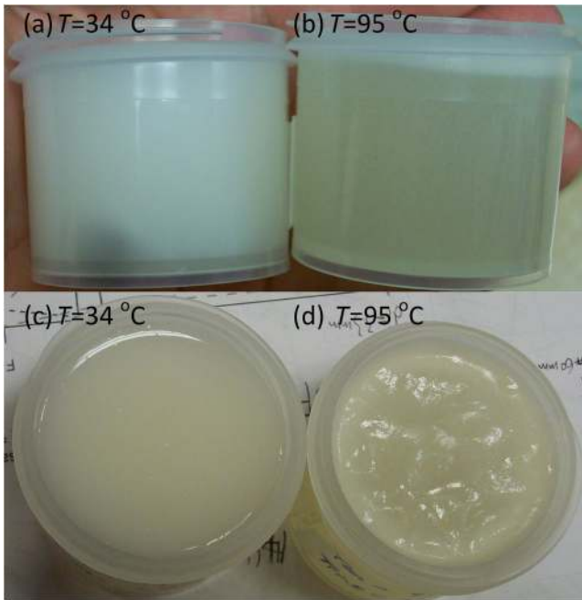
Fig. 7 Photographs of two solidified phantoms from Group 2, with the same mixing time length of 30 min but different mixing temperatures (34°C and 95°C, respectively), before they were removed from the sample molds. (a) and (b) are viewed from the side, while (c) and (d) are from the top.
