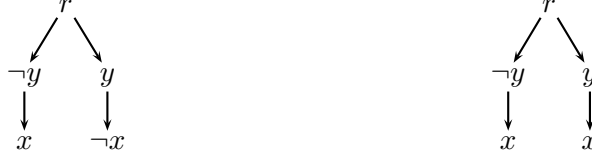
Figure 5.2: The two possible refuting assignment trees by Definition 5.3.3 for the unsatisfiable PCNF \psi := \exists y \forall x. (x \vee \neg y) \wedge (\neg x \vee y) \wedge (\neg x \vee \neg y) .
