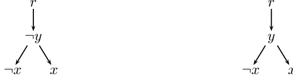
Figure 3.1: Two possible assignment trees of the PCNF \psi := \forall x \exists y. (x \vee \neg y) \wedge (\neg x \vee y) from Example 3.1.1 where y is erroneously assigned before x .
