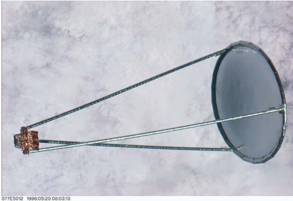
Figure 2.21: The 14 m diameter IAE reflector antenna in space (Courtesy of L'Garde, Inc.).
