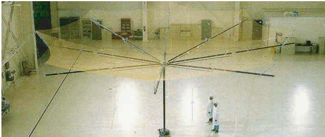
Figure 2.10: The 12 m diameter hinged-rib antenna for the ACeS system (Courtesy of Harris Corporation).
