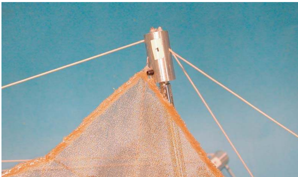
Figure 7.13: Cylindrical joint fitting with grub screw.
