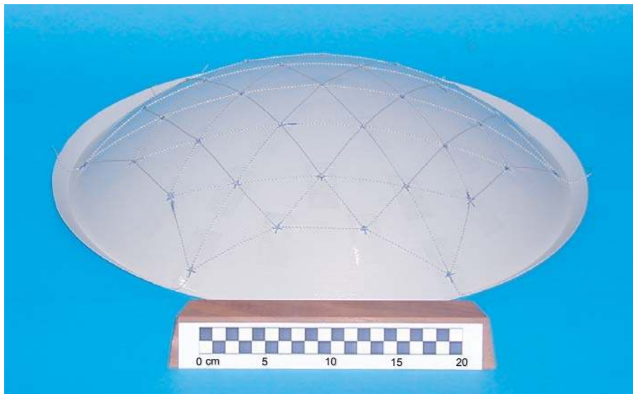
Figure 7.10: Paraboloidal plastic mold with the first of the two three-ring nets attached. The radial cables are used to connect the net to the ring structure.
