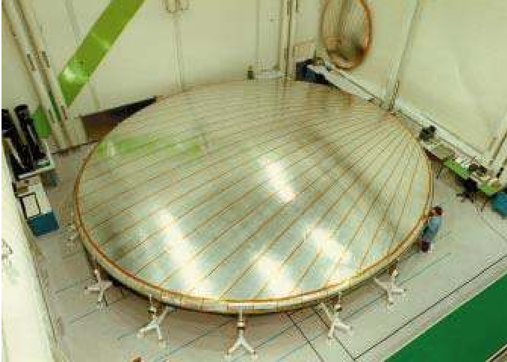
Figure 2.20: The 12 m diameter model of the inflatable space rigidised reflector antenna (Courtesy of A. G. Roederer, ESA).
