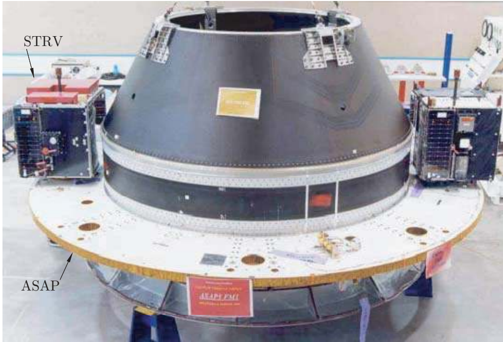
Figure 5.1: DERA's small satellites STRV-1 C and D on Ariane-5 ASAP for launcher fit check (Courtesy of DERA).
