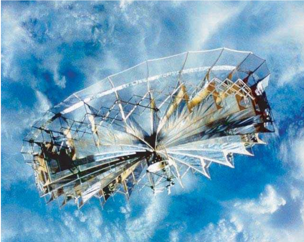
Figure 2.12: A 5.6 m diameter EGS antenna in space. Photo taken from the orbital station MIR on July 28, 1999 (Courtesy of Energia-GPI-Space, Ltd.).
