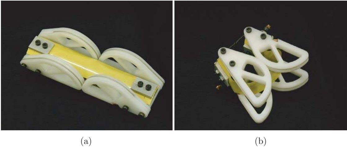
Figure 4.5: The tape spring rolling hinge: (a) deployed and (b) folded (Courtesy of A. M. Watt).
