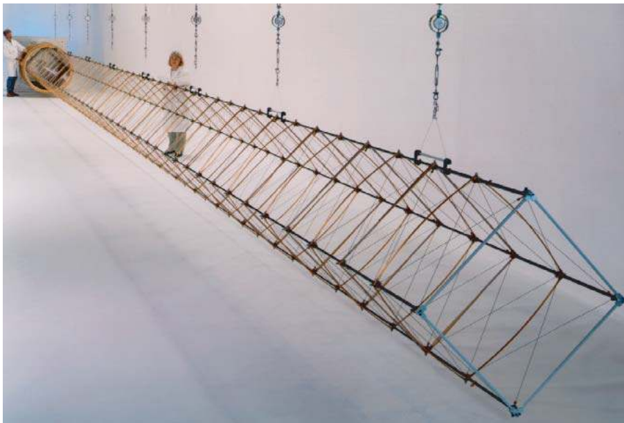
Figure 2.6: FAST mast for the ISS (Courtesy of AEC-Able Engineering Company, Inc.).
