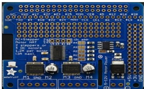
Figure 3. Stepper Motor Hat (Adafruit Industries, 2019, p.5)
