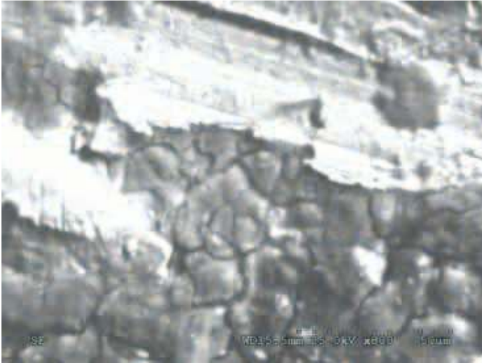
Figure 1 Liner lacquer deposit prior to acetic acid sprinkling
