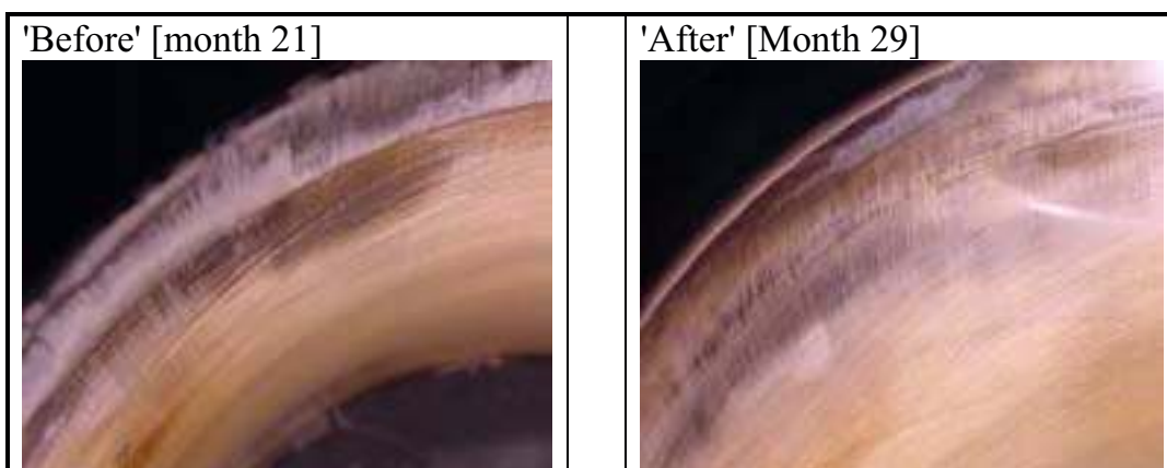
Figure 4-23 Cylinder B5 before and after 8 months fuel additive treatment. Lacquerish deposits replace the soot above upper ring reversal.
