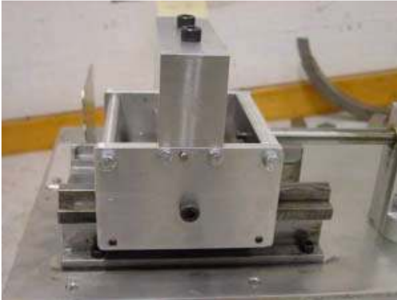
Fig 3. Rigid wagon carrying piston ring assembly
