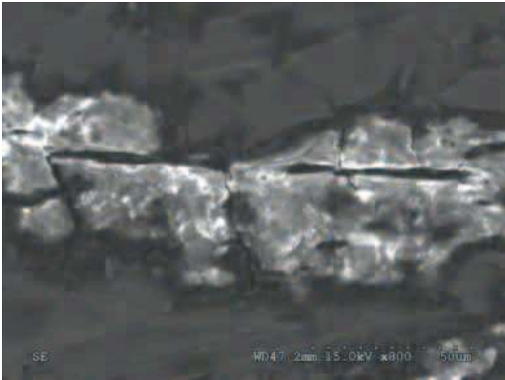
Figure 3-18 Lacquer with crack parallel with groove (center region)
