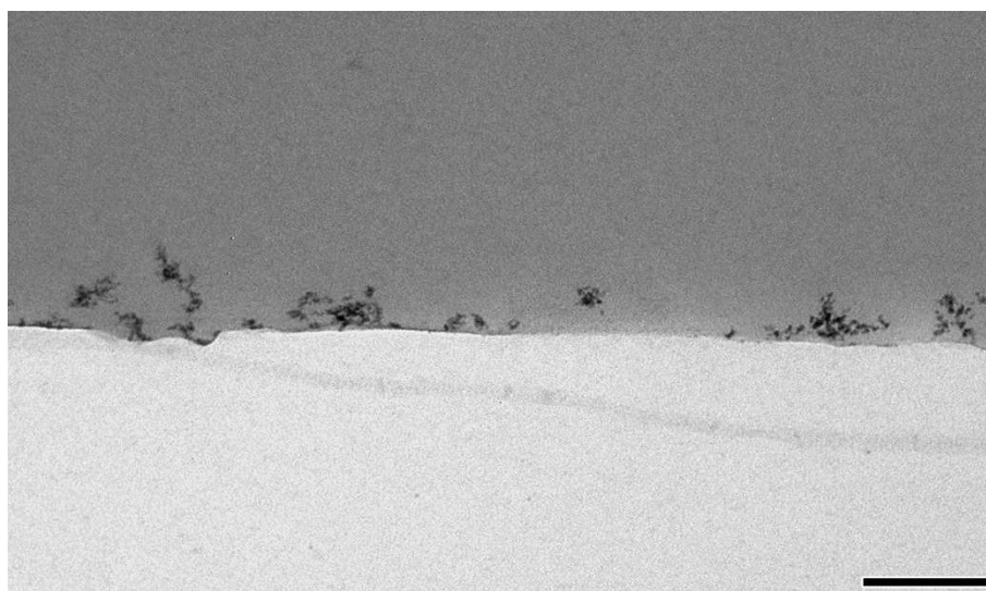
Figure 3 Nanoparticle morphology. Section profiles (transects) of TiO 2 nanoparticles collected from the aerosol on filters, embedded in Epon and cut perpendicularly to the filter. Note that the as 20 nm measured TiO 2 aerosol particles are already agglomerates of smaller primary particle structures of 3 - 5 nm formed immediately after spark ignition and condensation. Bar: 200 nm.
