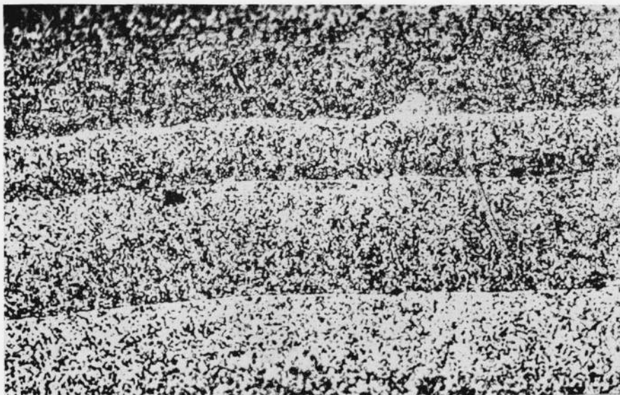
FIGURE 3. Electroless nickel deposit, after annealing at 800° C for ½ hr, showing apparent precipitation, ×500. Knoop hardness number 470.
