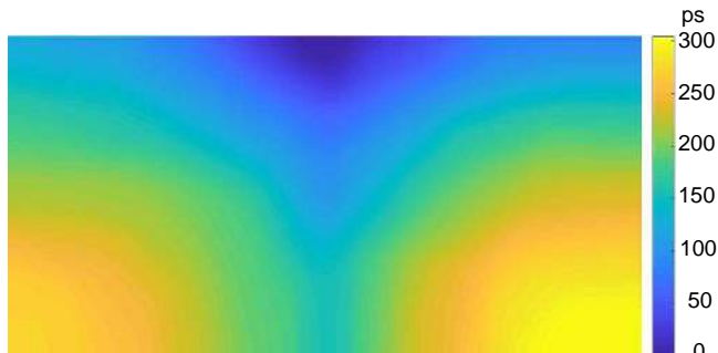
Figure 3. Calibrated spatial variant phase delay map.
