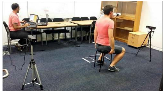
Fig. 1. The proposed system for performing PFT with 2 opposing Kinects.
