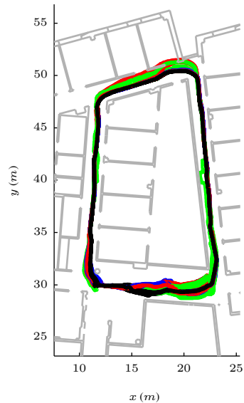
Fig. 6. Combined traces of all successful trials of all approaches: green (KR), red (KS), blue (KC) and black (FSPF). FSPF CGR localization is seen to have the least variation across trials.
