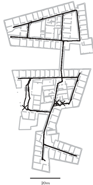
Fig. 9. Trace of robot location for the long run trial. The locations where localization had to be reset are marked with crosses.
