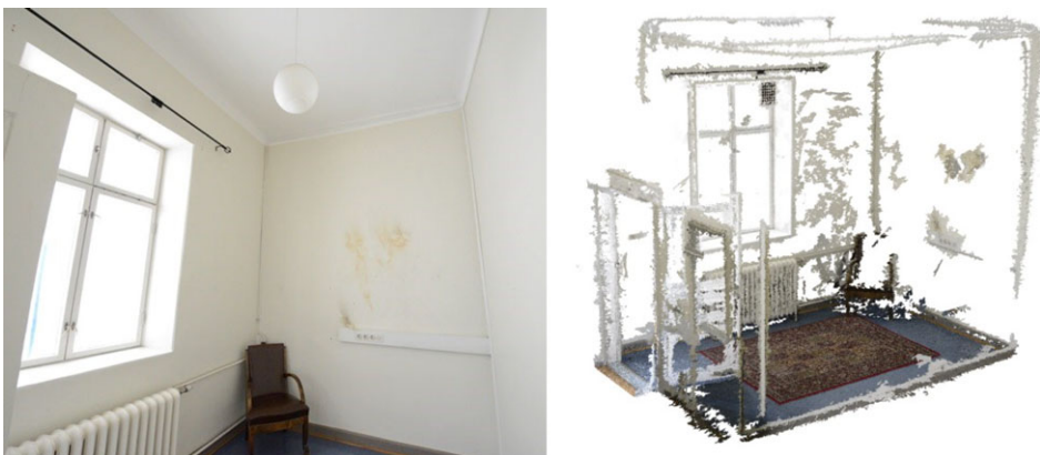
FIG. 1. Segment of an example image from an individual room (left). The white walls proved to be too featureless for image matching (right).
