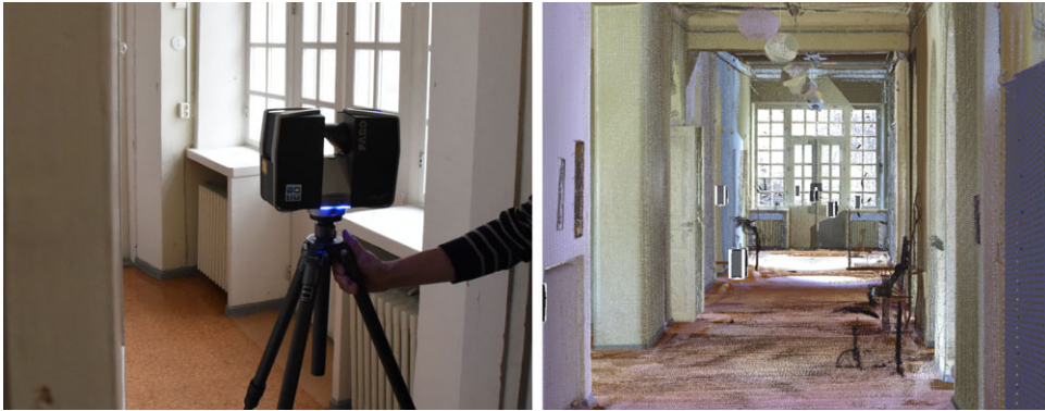
FIG. 3. Preparing to scan the main corridor of the building (left) and a coloured point cloud resulting from several co-registered scans (right).
