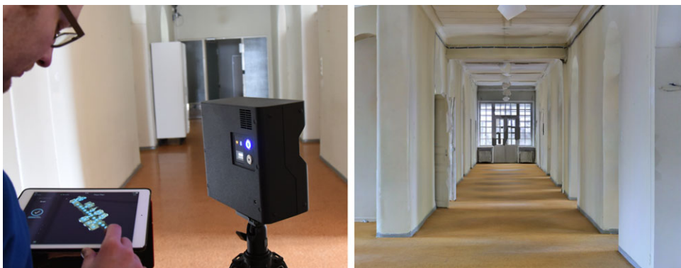
FIG. 2. Operating the Matterport system (left) and a segment of the completed textured model obtained from the cloud showing the end of the largest corridor (right).
