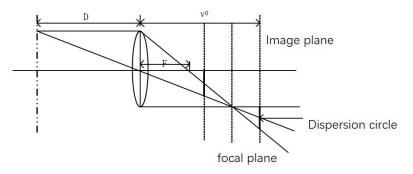
Figure 2. The geometric structure of real aperture imaging.
