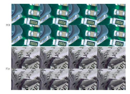
Figure 3. Registered defocused image sequence (partial), PCB and Alp.
