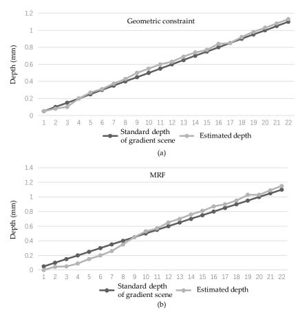
**Figure 7.** Gradient scene depth estimation quantitative comparison: (**a**) geometric constraint method; (**b**) MRF method.
