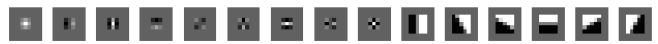
Figure 2: The filters used for computing texture variations and gradients. The first 9 are Laws' masks, and the last 6 are oriented edge filters.
