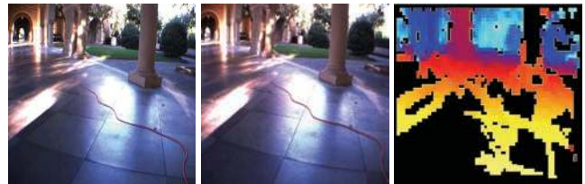
Figure 1: Two images taken from a stereo pair of cameras, and the depthmap calculated by a stereo system. Colors in the depthmap indicate estimated distances from the camera.
