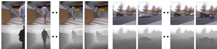
Fig. 1. Our technique takes a video sequence ( top row ) and automatically estimates per-pixel depth ( bottom row ). Our method does not require any cues from motion parallax or static scene elements; these videos were captured using a stationary camera with multiple moving objects.
