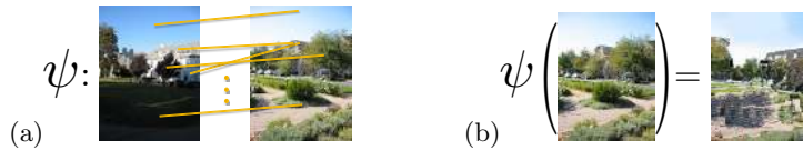
Fig. 3. SIFT flow warping. (a) SIFT features are calculated and matched in a one-to-many fashion, which defines \psi . (b) \psi is applied to achieve dense scene alignment.
