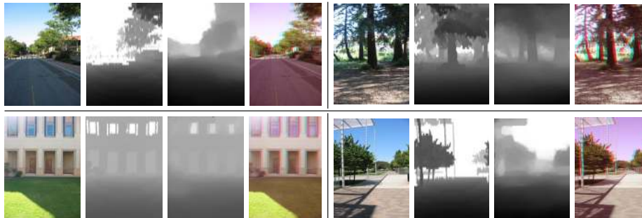
Fig. 8. Single image results obtained on test images from the Make3D dataset. Each result contains the following four images (from left to right): original photograph, ground truth depth from the dataset, our inferred depth, and our synthesized anaglyph image. The depth images are shown in log scale. Darker pixels indicate nearby objects (black is roughly 1m away) and lighter pixels indicate objects farther away (white is roughly 80m away). Each pair of ground truth and inferred depths are displayed at the same scale.
