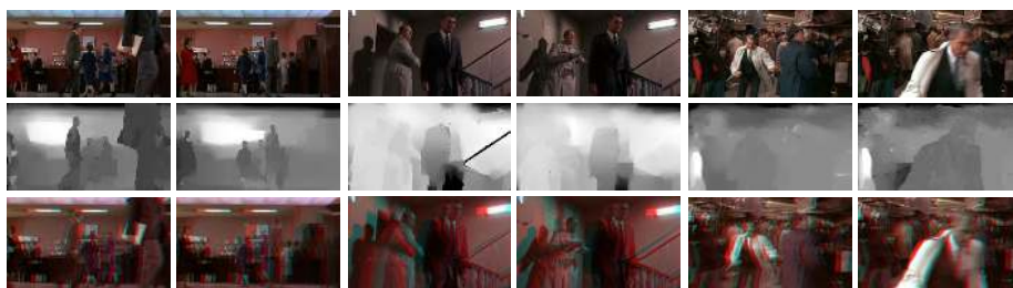
Fig. 11. Several clips from the feature film Charade . Each result contains (from top to bottom): the original frames, estimated depth, and estimated anaglyph image automatically generated by our algorithm. Some imperfections in depth are conveniently masked in the 3D image due to textureless or less salient regions.
