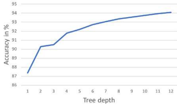
Fig. 11. Accuracy of the proposed machine learning invalidation. Notice how the accuracy rapidly increases up until a tree depth of 7, after which each level of the tree only marginally improves results.
