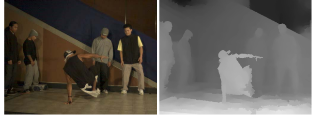
Fig. 1. Example texture image (left) and the corresponding depth image (right). A typical depth image contains regions of linear depth changes bounded by sharp discontinuities.
