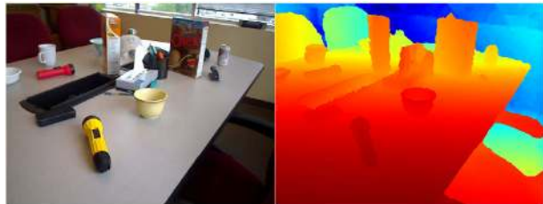
Fig. 1. RGB image (left) and the corresponding depth map (right) captured with a PrimeSense camera. The depth values go from small to large as the color changes from red to blue.
