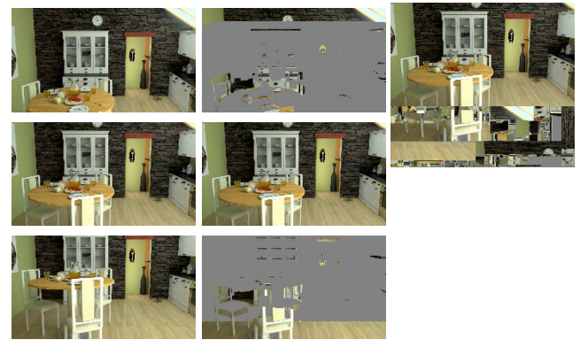
FIGURE 2. Inter-view redundancy removal using MIV: input views (left column), pruned input views (center column), and atlas containing all preserved (non-pruned) information from input views (right column).
