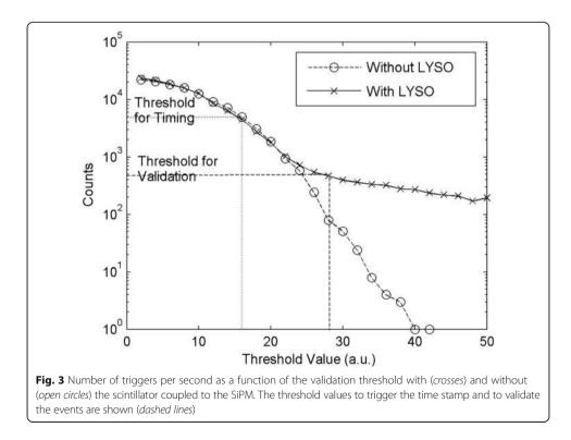
correspond to the actual SiPM dark count rate. The remaining dark count events that were greater than the validation threshold and that triggered the channel readout independently from a scintillation event were discarded in the post processing by the cluster finding algorithm and by the rule that more than three SiPMs had to belong to each of the accepted events.
