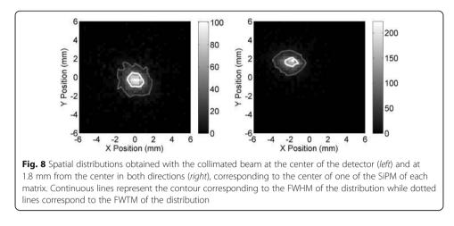
beam spot size. The distance between the center of the two distributions (at the center and at half the pitch) is 1.79 mm in the *X* direction and 1.92 mm in the *Y* direction, close to the expected value of 1.8 mm (half the pitch). This suggests that the width of the distribution obtained at the center of the detector is not distorted by the effects of the centroid algorithm used here. The reconstructed positions and width of the distributions are summarized in Table 1.
