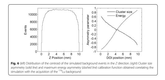
the cluster size asymmetry on the DOI position obtained correlating the simulation with the acquisition of the <sup>176</sup>Lu background, while the dashed line is related to the maximum energy asymmetry.
