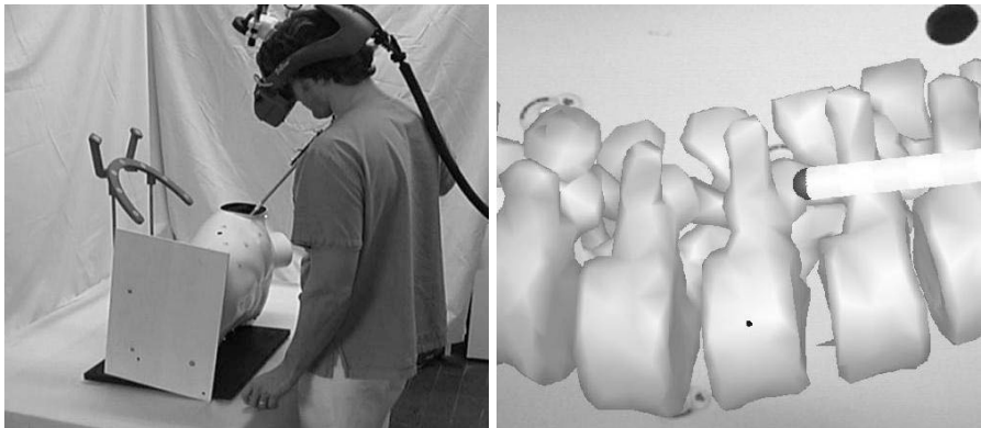
Fig. 2. Augmented surgical instrument serves as the pointer device. The small black point is visualized. The surgeons were asked to touch the point with its tip in the virtual position.
