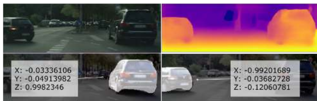
Figure 6: One benefit of our approach is that individual object motion estimates in 3D are produced at inference and the direction and speed of every object in the scene can be obtained. Predicted motion vectors normalized to unit vectors are shown (yaw, pitch, raw are not shown for clarity).
