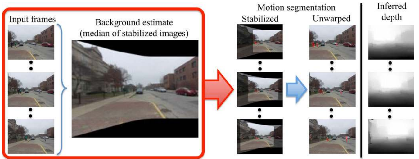
Fig. 6. Example of our motion segmentation applied to a rotating sequence. We first estimate homographies to stabilize the video frames and create a clean background image using a temporal median filter. We then evaluate our estimate of motion thresholding metric on the stabilized sequences, and unwarped the result (via the corresponding inverse homography) to segment the motion in the original sequence. We can then improve our inferred depth using this segmentation. Note that this technique is applicable to all video sequences that do not contain parallax induced from camera motion.
