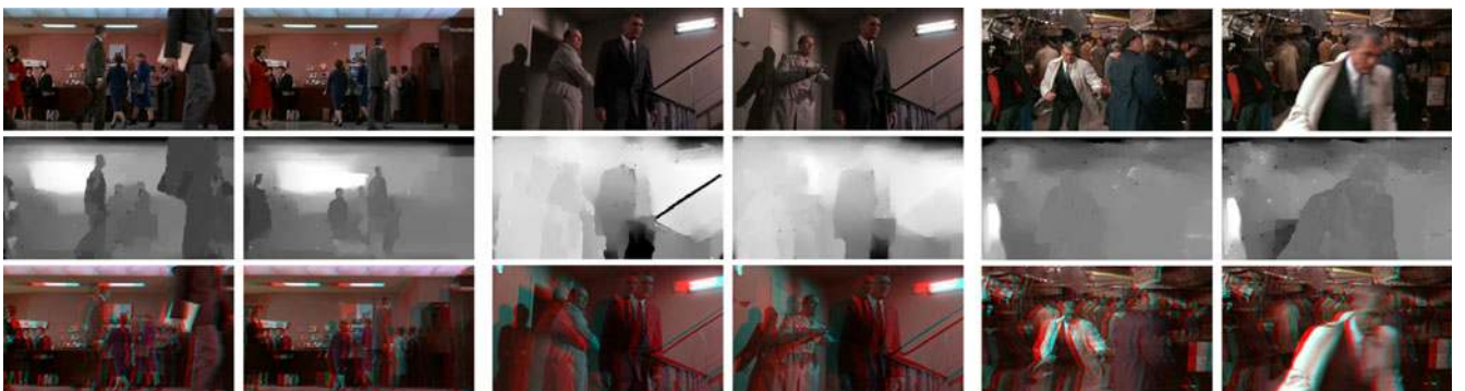
Fig. 17. Several clips from the feature film Charade . Each result contains (from top to bottom): the original frames, estimated depth, and estimated anaglyph (red/cyan) automatically generated by our algorithm. Some imperfections in depth are conveniently masked in the 3D image due to textureless or less salient regions.
