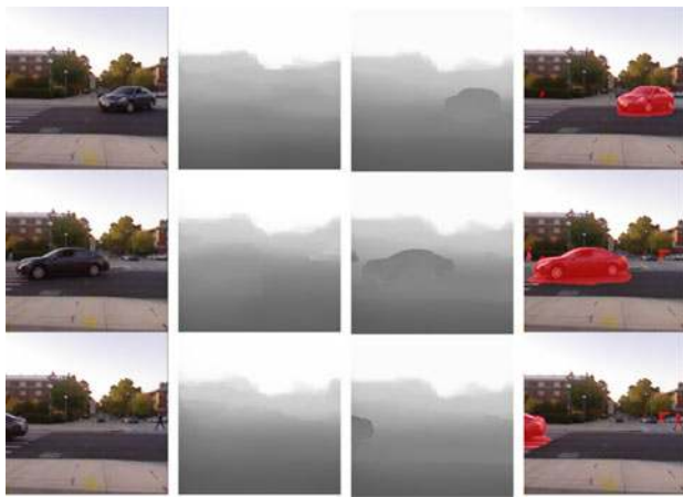
Fig. 5. Importance of temporal information. Left: input frames. Mid-left: predicted depth without temporal information. Note that the car is practically ignored here. Mid-right: predicted depth with temporal information, with the depth of the moving car recovered. Right: detected moving object.
