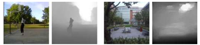
Fig. 20. Example failure cases. Left: thin or floating objects (pole and basketball) are ignored. Right: input image is too different from training set.
