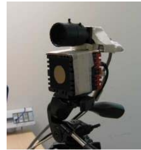
Fig. 10. Experimental setup for the proposed method. The capturing system consists of a “Point Grey Flea” color camera and a “Mesa Imaging SR4000” depth sensor.
