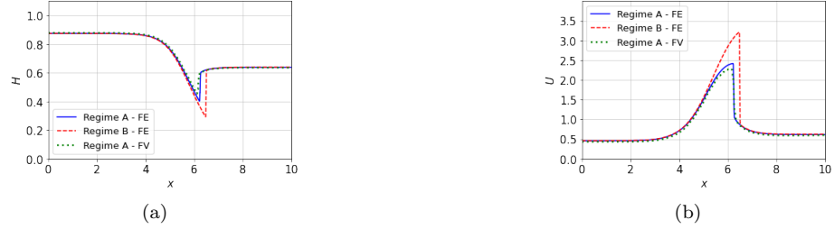
Figure 15: Comparing fluid elevation H (a) and mean velocity U (b) for regime A and B at t = 10s . The difference between the two regimes is evident where the slope is changing.
