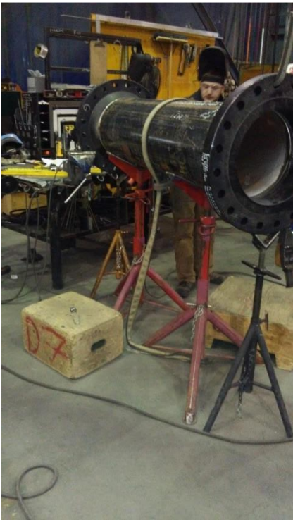
Figure 15: Pipe loaded at a fitting station for being assembled
