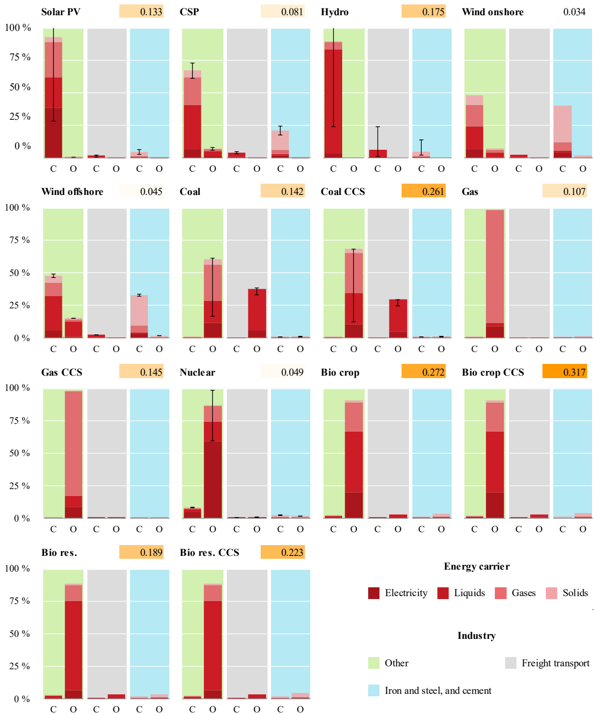
Fig. 3. Life cycle indirect energy requirements for 14 main types of power generation for Europe and year 2010, broken down into phase (construction and end-of-life total, denoted by C; operational, denoted by O), energy carrier used (electricity; liquid, gaseous and solid fuels) and industry in which the use occurs (iron and steel; cement; freight transport; and other). Stacked columns represent relative contributions to total indirect energy (i.e., sum across all columns and stacked categories within columns equals 100% for each plot). For bio crop, results for a scenario assuming no restriction on types of cellulosic biomass crop available and where irrigation is allowed are shown as an example (the ‘TAX30_begr_bet_ir’ scenario’; see electronic supplement). Error bars indicate extrema totals across technology subcategories relative to the mean across technology type (cf. Table 1). Vertical axes are cut at 100%, but some maxima lie above 100%: slightly >100% for solar PV, C, other; and 350% for hydro, C, other. Numerical values above plots give total indirect energy requirements in units of megajoule (MJ) energy input per MJ electricity output and exclude losses in the power production process itself. The values are shaded according to their relative magnitude (in reference to the whole set of values), with light
