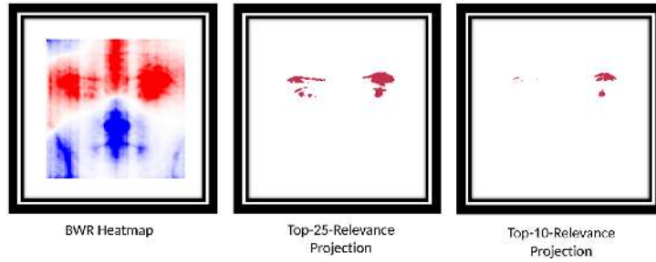
Figure 3: Heatmap produced based on a BWR color scheme (left) compared to reduced heatmap only showing most relevant features that aggregate 25 % (middle) and 10 % (right) of the relevance mass present in the corresponding relevance map (shown prediction is for AU02, the “outer brow raiser”)
