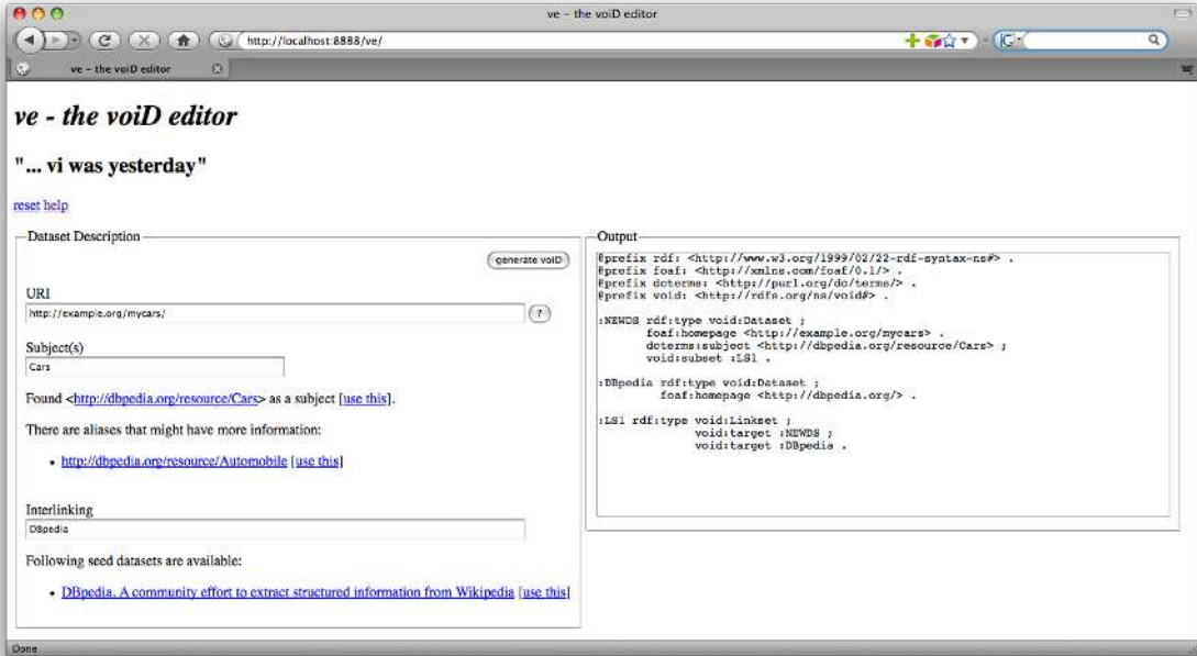
Figure 5: Manual creation of void descriptions with ve .
