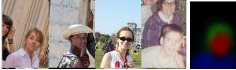
Figure 5. Left: Examples of a poselet. Right: The poselet soft mask for the hair, face and upper clothes.
