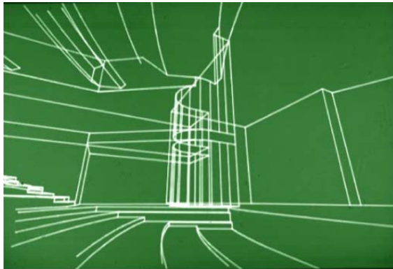
FIG. 7: One version of the main hall of Helsinki opera house (architects Hyvämäki - Karhunen - Parkkinen) modelled with Proj-program by Tapio Takala et al. 1978-84. An early example of free architectural forms expressed with CAD. Straight and curved lines could be modelled spatially in 3D, though yet without volume modelling.
