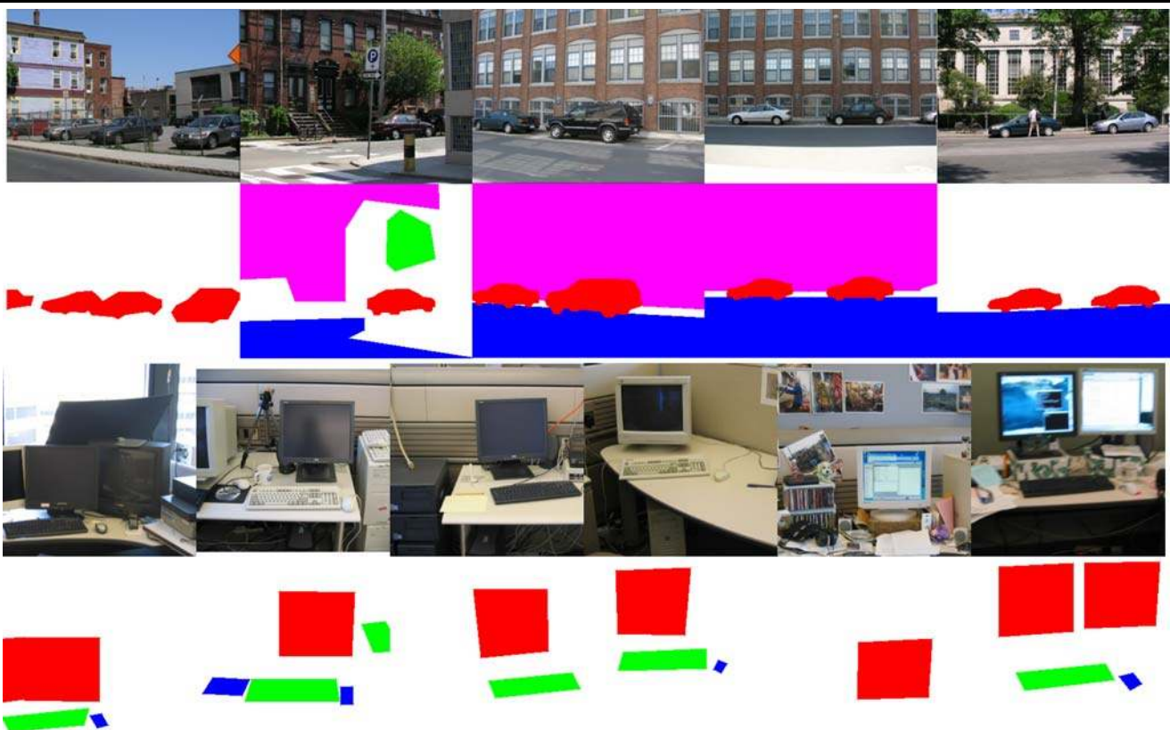
Fig. 4 Scale-normalized images used to evaluate two-dimensional models for visual scenes, available from the MIT LabelMe database (Russell et al. 2005). Top : Five of 613 images from a partially labeled dataset of street scenes, and segmented regions corresponding
