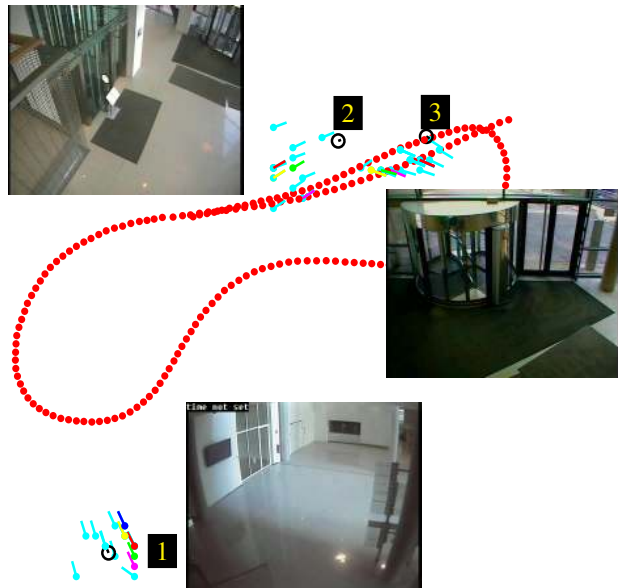
Figure 10. Localization of surveillance cameras. Small circles depict positions estimated from manually established point correspondences. Short lines with dots are the best fifteen (in order red, green, blue, magenta, yellow, cyan) returned virtual cameras obtained with the proposed method.
