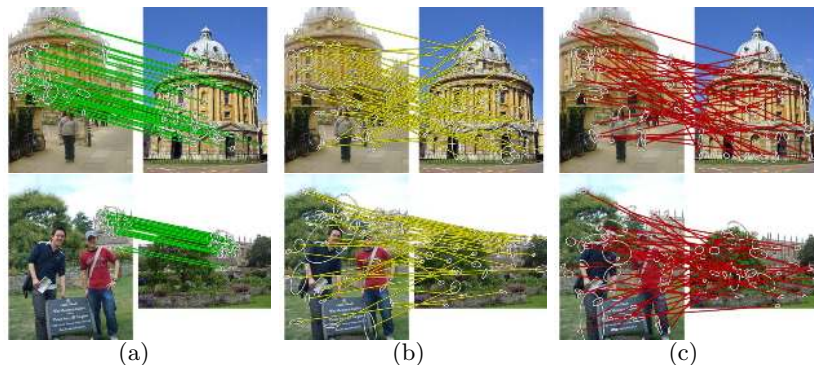
Fig. 1. Gathering training point pairs. Three groups of point pairs are shown: (a) inliers to an affine homography found using RANSAC (positives); (b) outliers which are nevertheless nearest neighbors in SIFT space (nnN); and (c) random pairs of points which are usually distant in descriptor space (ranN).
