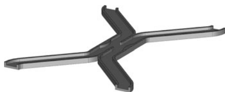
Fig. 5. CAD model for simulation including waveguide test fixture.
