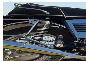
Fig 1.1:- Rear shock absorber and spring of a BMW R75/5 motorcycle
