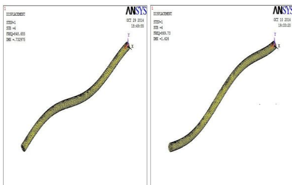
Fig 4.4 Comparison of fourth set of natural frequency analysis for steel and composite
