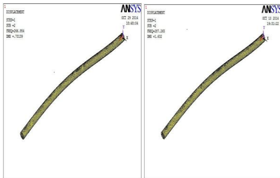
Fig 4.4 Comparison of second set of natural frequency analysis for steel and composite
