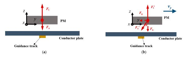
**Figure 2.** Guidance force analysis under different conditions: (**a**) PM and track are in alignment; (**b**) The vehicle exists in transverse displacement.
