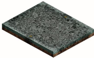
Figure 2. Meshed model of heat sink
