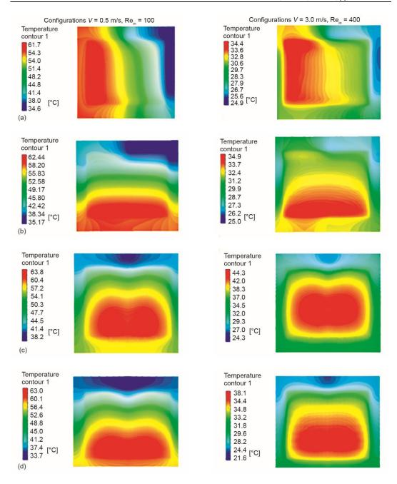
Figure 7. Temperature contours of hot surface of liquid cooling plate at different Reynolds numbers; (a) parallel-I, (b) parallel-II, (c) distributor-I, and (d) distributor-II (for color image see journal web site)
