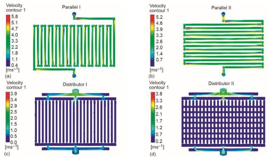
Figure 4. Channels' average velocities in different flow configurations (for color image see journal web site)
