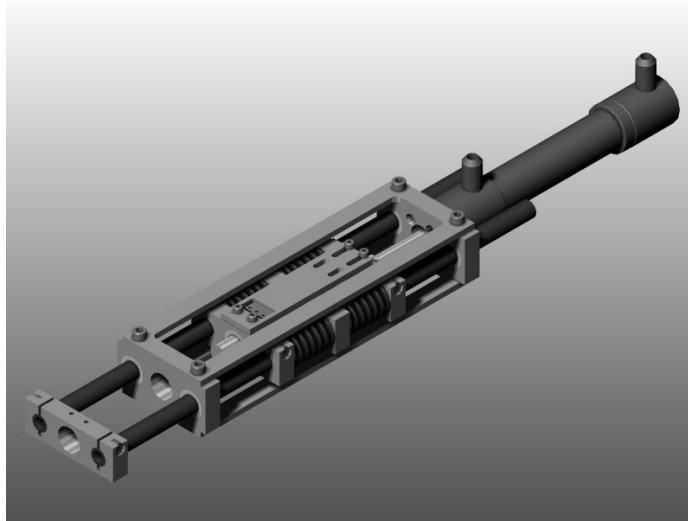
Figure 4-1: Prototype Actuator CAD model. A 20MPa pressure source is connected to a MOOG series 30 flow control servo valve (not shown) that directs flow to the two chambers of the hydraulic cylinder. The piston is coupled to the output through four die compression springs. The spring compression is measured with a linear potentiometer which implies force. A closed-loop controller actively moves the piston to maintain a desired spring deflection.
