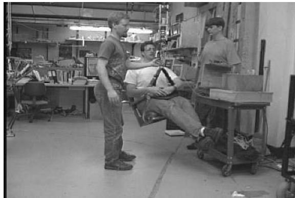
Figure 5-19: Fully loaded actuator demonstrating small force sensitivity. The actuator is fully loaded with 300 lbs and has a force equal to gravity pull on the load mass. Finger force of approximately 1 lb can get the actuator to move up and down. This shows that the dynamic range of the actuator is 300:1.
