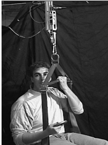
Figure 4-15: Risky testing the hydro-elastic actuator. The author is suspended under the hydro-elastic actuator. The actuator is supporting the load by a commanded force 1 lb above the downward force of gravity ( \sim 250lbs ). The author is holding a 2lb weight which drops the actuator. Releasing the weight causes the actuator to rise. The minimum resolvable force is 1 lb and is due to the noise floor of the sensor.
