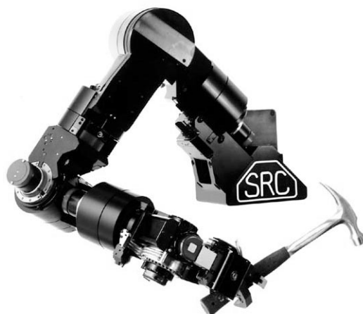
Figure 2-7: Sarcos Dextrous Arm. It is a hydraulic force controlled teleoperated manipulator that has been used for many applications including production assembly, undersea manipulation and hazardous material handling. The manipulator actuators have accumulators on either side of the hydraulic fluid chambers. This gives the actuators intrinsic compliance. Reprinted by permission of Sarcos.
