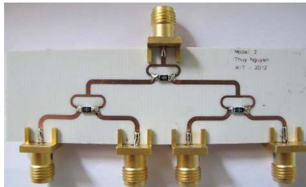
Fig. 5.17.: Fabricated circuit of the 4:1 Wilkinson Power Divider
